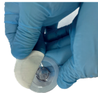
Remove the cover of the \varnothing 10 mm striker and fix it on the \varnothing 10 mm vial of the hardener. Remove the striker pin protection.
