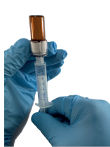
Attach the syringe by screwing it onto the hardener tip. Take up all of the hardener by sucking up with the syringe. Screw the syringe onto the base and inject the hardener. Mix by sucking up the contents of the mixture. Unscrew the Vial syringe from the base.
