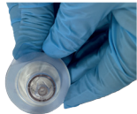
Remove the cover of the \varnothing 20 mm striker and fix it on the \varnothing 20 mm vial of the base. Remove the striker pin protection.
