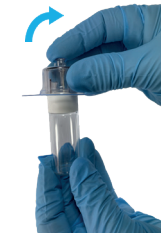
Remove the cover of the \varnothing 20 mm striker and fix it on the \varnothing 20 mm vial of the base. Remove the striker pin protection.
