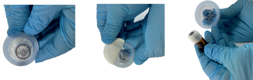
Remove the cover of the Ø10 mm striker and fix it on the Ø10 mm vial of the hardener. Remove the stricker pin protection.
