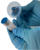
Remove the cover of the \varnothing 20 mm striker and fix it on the \varnothing 20 mm vial of the base. Remove the striker pin protection.
