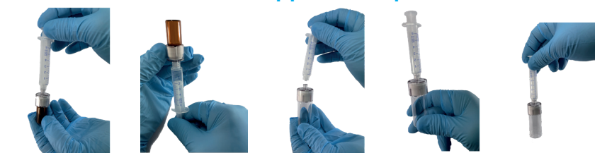
Attach the syringe by screwing it onto the hardener tip. Take up all of the hardener by sucking up with the syringe. Screw the syringe onto the base and inject the hardener. Mix by sucking up the contents of the mixture. Unscrew the Viale syringe from the base.
