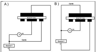
The measurement method used consists in applying a direct voltage U across the terminals of the sample and measuring the current I traversing it after a defined period of time (1 minute) in order to deduce a resistance R.
