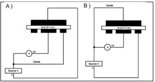
The measurement method used consists in applying a direct voltage U across the terminals of the sample and measuring the current I traversing it after a defined period of time (1 minute) in order to deduce a resistance R.
