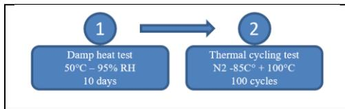
Samples were composed of an assembly of two 2024-T3 alloy plates coated with MAP® EPOX BLACK ESD and bonded with Redux® 312/5 adhesive. The size of the samples was 105 mm x 25 mm with a thickness of 1.6 mm
