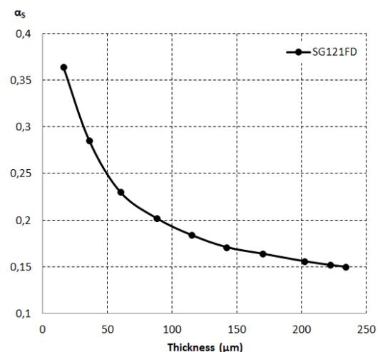
Figure 6 Evolution of solar absorptance of SG121FD versus thickness
