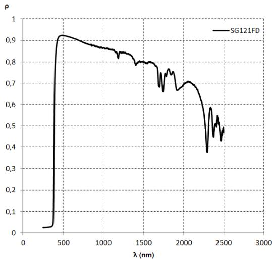
Figure 4 Reflectivity versus wavelength for SG121FD
