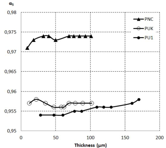
Figure 5 Evolution of solar absorptance of PU1, PUK and PNC versus thickness
