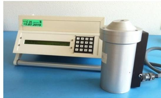
Figure 1 EL511 portable reflectometer
