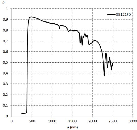
Figure 4 Reflectivity versus wavelength for SG121FD
