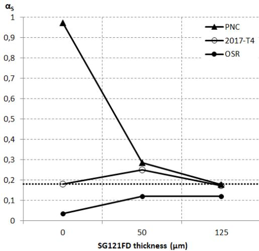
Figure 7 Evolution of SG121FD solar absorptance applied on different substrates
