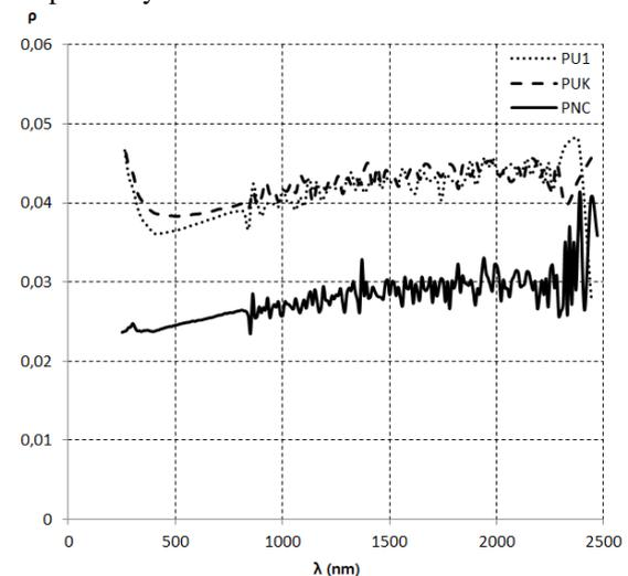
Figure 3 Reflectivity versus wavelength for PU1, PUK and PNC
