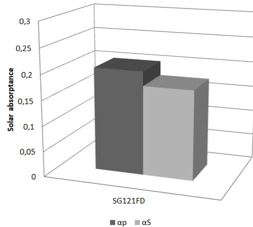
Figure 9 Comparison of solar absorptance measurement using a spectrophotometer and a comparative method (portable device) for SG121FD
