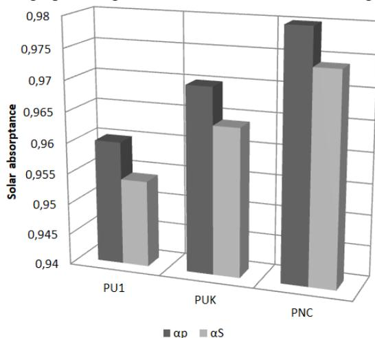
Figure 8 Comparison of solar absorptance measurement using a spectrophotometer and a compara-
